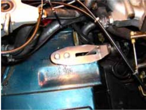
5. Now, focus on the accelerator lever on the fire wall which is now free as you removed the original linkage from it. Place the accelerator bracket from the kit over the lever so that the lever protrudes through the slot in the bracket.
