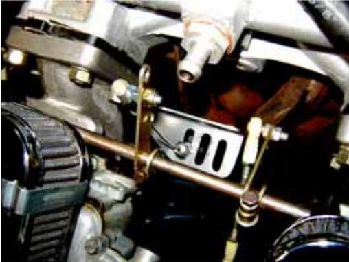
12. From the accelerator bracket end, slide the cable through the sleeve and attach the fitting to the accelerator lever with the clevis pin and snap ring.
